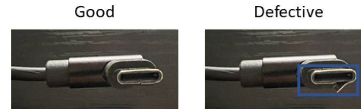
FIGURE 3.8 A learning data set aimed at detecting a common defect .
