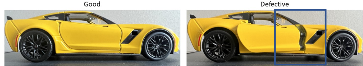
FIGURE 3.6 A learning data set aimed at detecting misalignments (e.g., in the car body).
